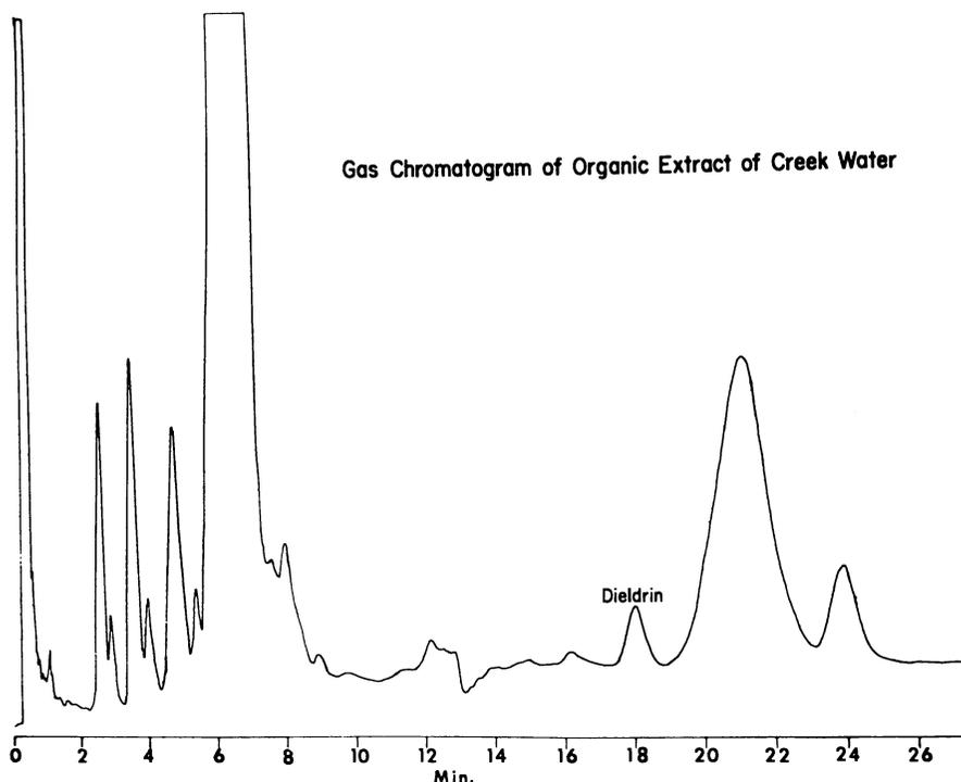
Figure 8. Gas chromatogram (FID) of a water extract containing dieldrin—ready for GC-MS analysis
