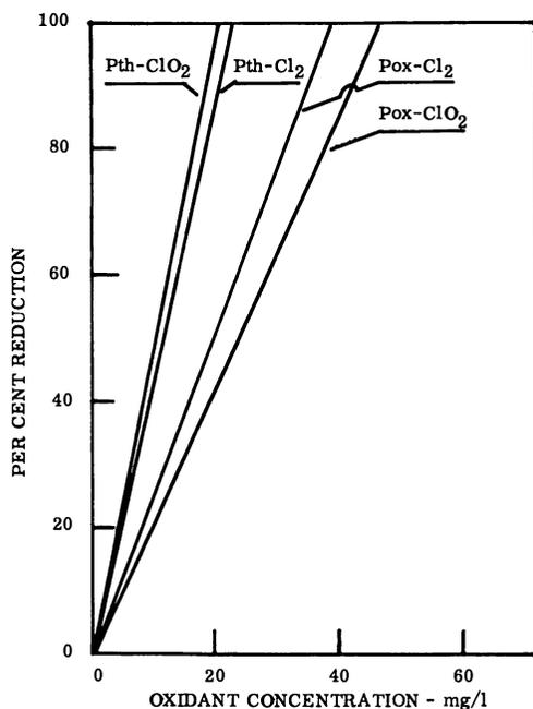
*Figure 3. Oxidation of parathion and paraoxon by chlorine and chlorine dioxide*
