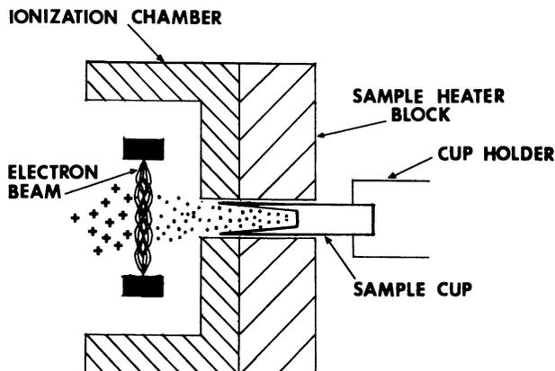
Figure 4. Direct inlet sample introduction system for a mass spectrometer
