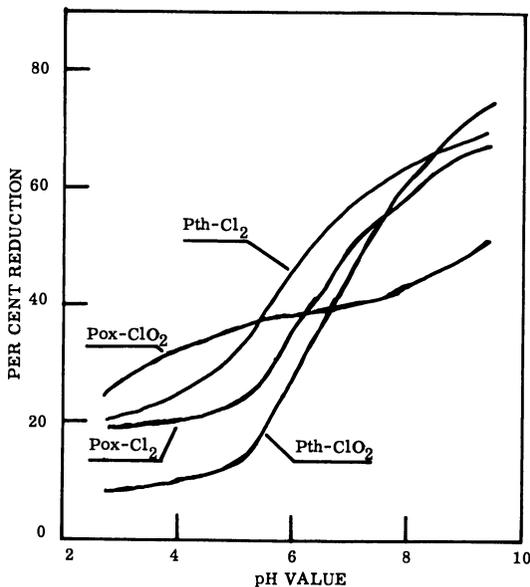
Figure 4. Effect of pH on the oxidation of parathion and paraoxon by chlorine and chlorine dioxide
