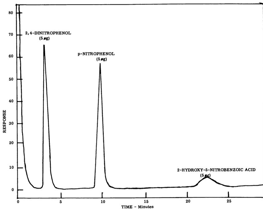
Figure 2. Isothermal separation of *p*-nitrophenol and some intermediate oxidation products
