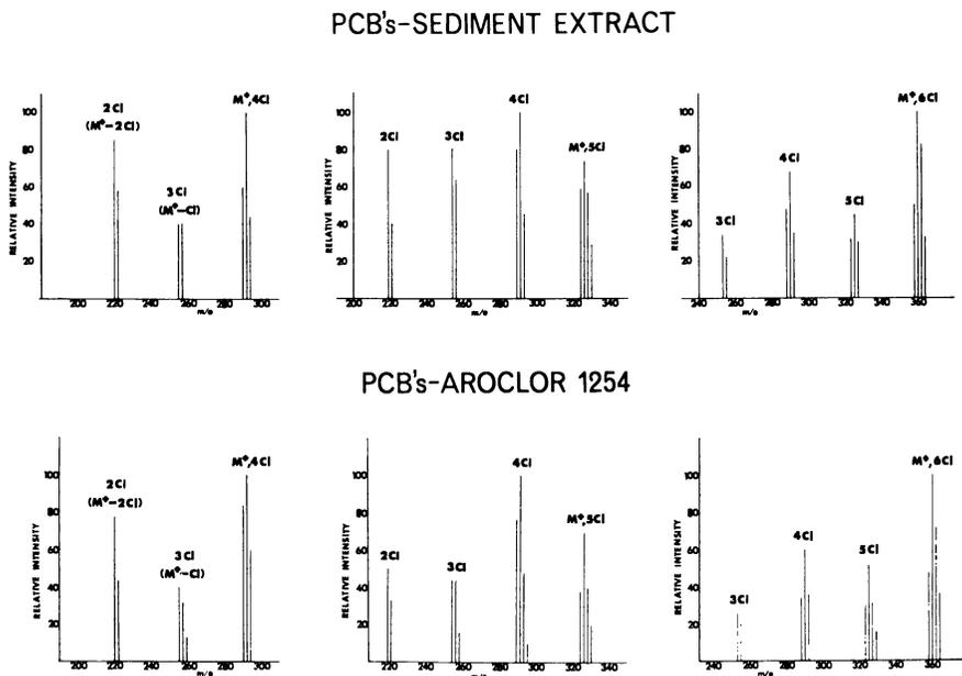
Figure 12. Partial mass spectra (GC-MS) of some of the PCB's of Figure 11 showing the number of chlorine atoms on each ion
