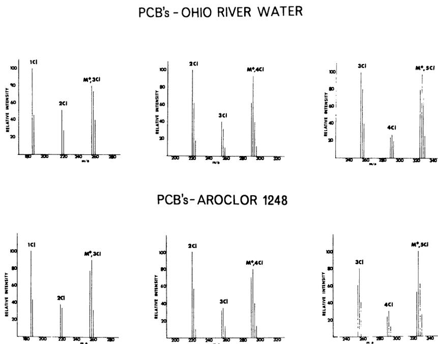
Figure 15. Partial mass spectra (GC-MS) of some of the PCB's of Figure 14 showing the number of chlorine atoms on each ion
