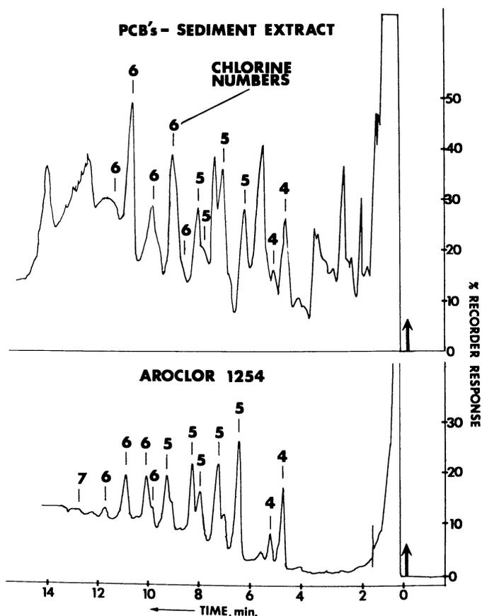
Figure 11. Gas chromatograms (FID) of polychlorinated biphenyls from the environment and in an Aroclor standard. (GC conditions are the same.)
