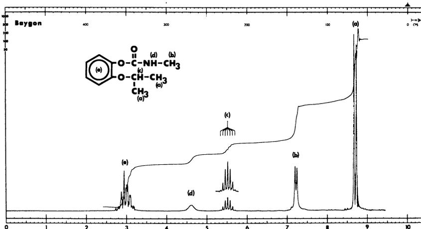
Figure 16. The 100 MHz NMR spectrum of Baygon in  $CDCl_3$ .
