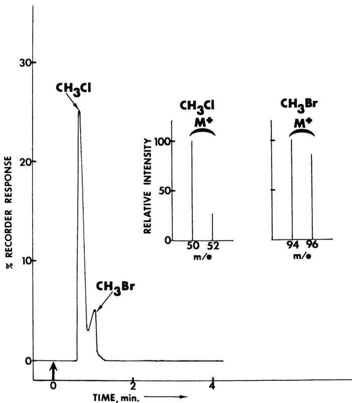
Figure 7. Gas chromatogram (FID) and partial mass spectra (GC-MS) of methyl chloride and methyl bromide in stored flour head gas
