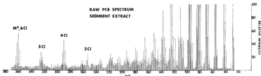
Figure 13. A mass spectrum (GC-MS) of a PCB in an environmental sample extract before background subtraction and normalization. The parent ion ( $M^+$ ) and fragment ions containing three, four, and five chlorine atoms gave discernable peaks.
