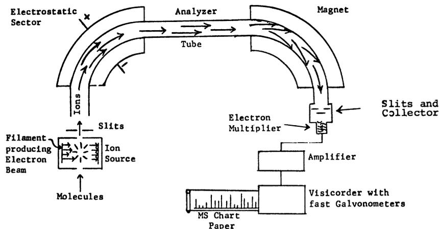
Figure 1. Block diagram of a double-focusing mass spectrometer
