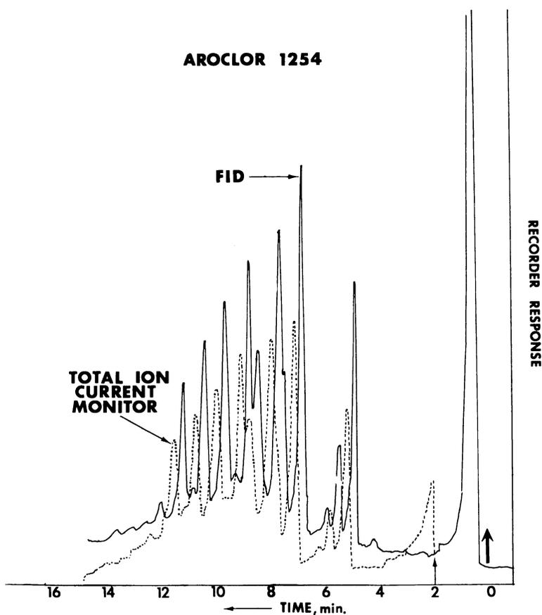
Figure 6. Dual pen recording of mass spectrometer total ion current monitor response and corresponding flame ionization detector response—Aroclor 1254. (Recorder pens are displaced slightly.)
