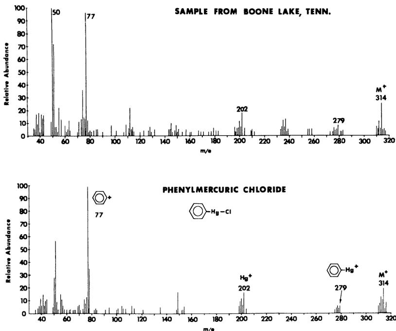
Figure 3. Mass spectra of phenyl mercuric chloride
