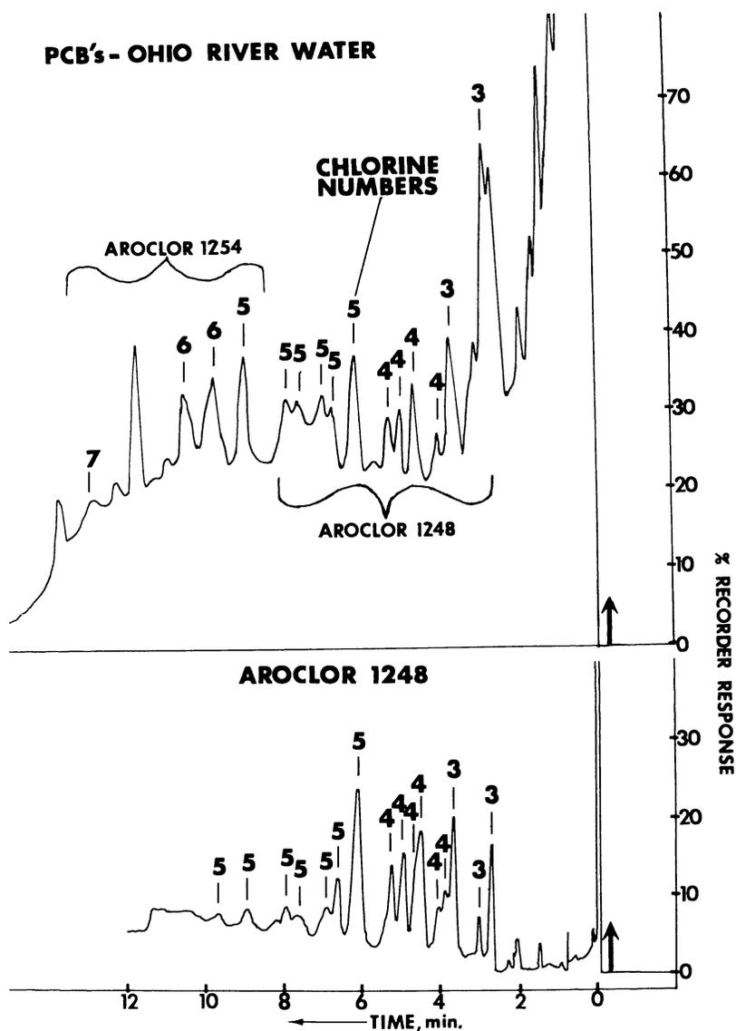
Figure 14. Gas chromatograms (FID) of PCB's in a river extract and in an Aroclor standard. (GC conditions are the same.)
