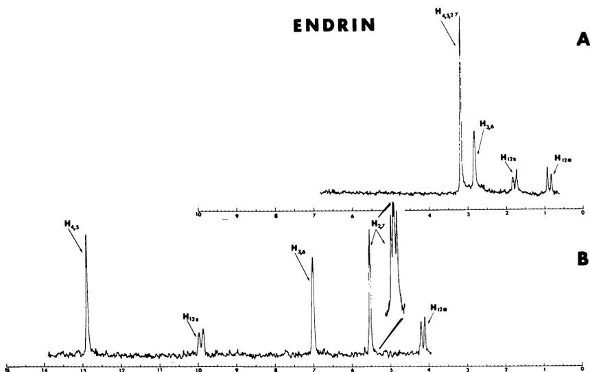
Figure 18. The 100 MHz NMR spectra of (A) endrin (0.14 M) without  $\text{Eu(DPM)}_3$  and (B) with 0.07 M  $\text{Eu(DPM)}_3$  in  $\text{CCl}_4$ .
